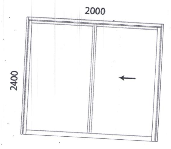
Aluminum – Glass Sliding Door Standard sizes: 2100mm and 2400mm high, widths of 2220mm, 2670mm,3120mm and 3570mm.
