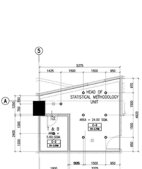
10 22F HEAD OF STATISTICAL METHODOLOGY UNIT REFLECTED CEILING PLAN
